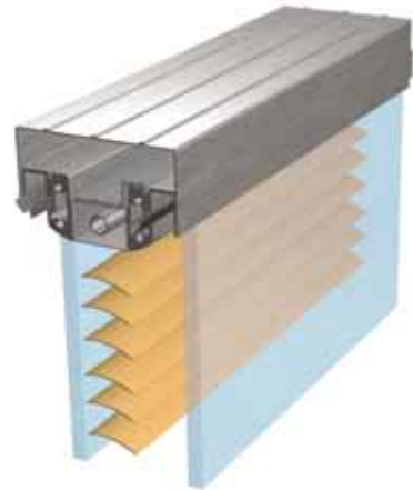
Ovation recessed blind channel detail
